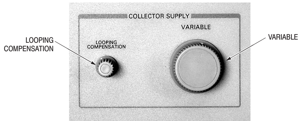
Figure 2–6: Collector Supply controls
